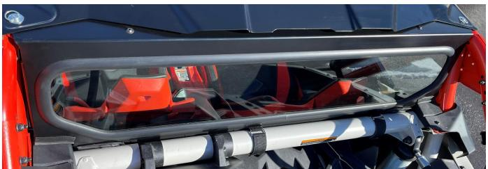
\*\*Installation Hint\*\* The edge seal bulb may not be pushed tight onto the frame in some areas because of shipping. Push seal on as tight as possible before installing. Once installed the bulb will stay tight because of contact with the plastic parts on the X3.
