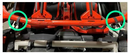
**Step 3.** Once in place insert the straps in the top slots from the rear of the machine with the Velcro side facing up. Rout the straps back out the lower slot and underneath the cross tube on the frame. The metal ring should be on the back side (outside) of the windshield. Loop the straps around and through the metal ring and pull tight. Tighten the straps and make sure the windshield is pulled towards the lower rear bar.
