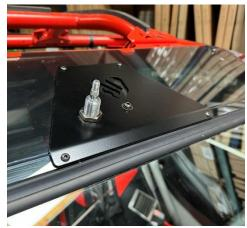
When all holes are drilled, place box with motor in place with the large shaft going through the large hole. Secure in place with the large nut, and the 6mm bolt with lock washer and washer.
