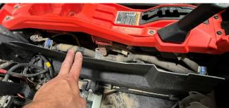
Install switch by taking out block off insert that comes on the X3 where you want the plug. Un-plug switch from harness and feed switch wiring through desired switch opening. Plug switch back in (It is directional and will only line up one way. Be careful not to try to force it the wrong way.). Push switch into place till it clips in.
