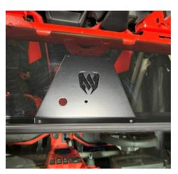
With mount plate bolted on, use a 3/16 drill bit to drill out the top two mount plate hole through the polycarbonate visor. Use a ¼" drill bit to drill out the medium size hole near the middle of the plate. Use a ¾
