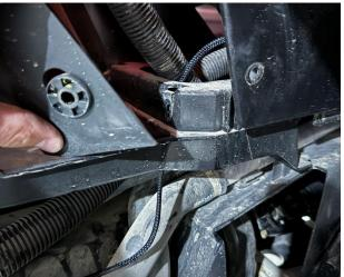
Locate the 3 power posts under the red rubber cover. The top post is ground. The middle post is always on power. The bottom post is key on power. Connect the black wire to the top post by removing the nut and putting the wire on and re installing the nut. Attache the red wire to the BOTTOM post for Key on only power
