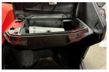
Next, open the glove box and remove the two bolts along the front edge of the dash shown in picture above. Pull away those plastics to continue running the harness behind the plastics. Leave harness hanging out jus left of the glove box.
