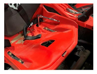
With seat out, Remove the one torx bolt circled in the picture below. Pull out at the top of the black side plastic panel to release clips and lift panel out of place.
