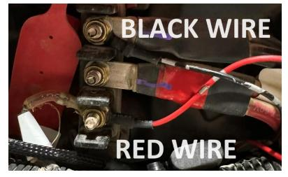
At this point test to make sure the switch and motor work by turning machine on (doesn't need to be running) and testing for power at the switch, and that the motor runs when switch is turned on. This is also important to do to make sure the motor is in the parked position for wiper arm installation. The motor will always return to the parked position when switch is turned to park. Reinstall all covers, hardware, and seat.
