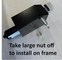
**Step 2: Install wiper Motor onto windshield**. Use a 1/8 Allen key and a 3/8" wrench/socket to Remove the two center bolts on the visor that bolts into the windshield frame. Place mount plate (plate with logo) onto visor with two bottom holes lining up with the two holes you removed the bolts from. Use two of the new longer bolts to fasten mount plate to windshield visor and frame.
