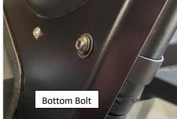
After all bolts have been started loosely, adjust windshield position and tighten all mounting hardware.
