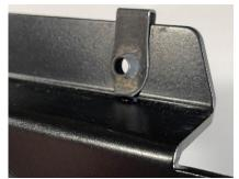
**STEP 1**. Install Clip-Nuts onto the top of the windshield frame as shown in pictures above, (this step may have been completed before shipping) The threads should be on the front side of the windshield.
