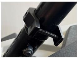
**STEP 3**. Place windshield on RZR and secure with provided hardware. Use the .75" long bolts (with flat washer and lock washer) on the top by bolting from the inside of the rzr through to the clip-nuts. Then use the .5" Long bolts (with flat washer and lock washer) on the bottom mounts bolting from the front into the threaded
