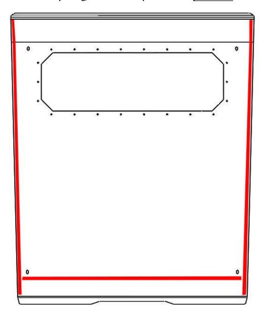
**STEP 2**. Place the roof on the top of the cage lining up each hole. Start the  $\frac{3}{2}$  bolts with washers and nuts in each available hole. Begin tightening the bolts starting at the back making sure to keep the roof centered.
