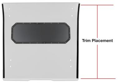
**STEP TWO –** Place the roof on the top of the cage lining up each hole. Start the 3/4 " bolts with washers and nuts in each available hole. Beginning tightening the bolts starting at the back making sure to keep the roof centered.
