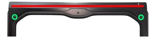
**Step 1:** Bolt the Windshield attachment to the windshield using the two  $\frac{1}{4}$ -20 x  $\frac{5}{8}$ " bolts with washers on both sides. Circled in green above is where the  $\frac{1}{4}$ -20 x  $\frac{5}{8}$ " bolts go.
