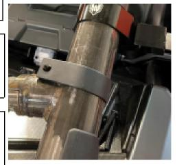
**Optional step:** Apply adhesive foam to anywhere that the roof contacts the windshield to prevent rattling. Approximate location of foam is in the picture in red.
