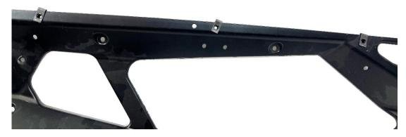
Carefully place door skin on factory door frame and slide the top mounting bracket over the top edge of frame. First insert two ½" bolts with washers into the two threaded spacers. Start with these two bolts because they have the least amount of adjustment. Leave bolts loose enough to be able to move skin to help align other bolts. (Use a 5/32 Hex/Allen key on these bolts)
