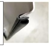
**STEP 3.** Mount door onto factory Frame. Install 3 clip-nuts onto the top edge of door frame as shown below. Make sure the threaded side is on the outside of the frame.
