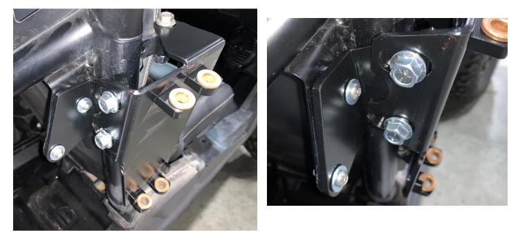
The doors may already have the hinge-pin plates loosely installed in the doors. Carefully install each door by setting it on the mounts aligning the pins with the holes on the b pillar mounts. The doors must be open about ¾ of the way to clear the hold in stops. Make sure the door has settled all the way into the pins before closing. If the doors are not in all the way they won't close and may cause damage if you force them to close.
