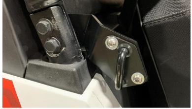
Step . Install B-Pillar mounts on each side as shown leaving bolts loose for adjustment. If you have a stock cage use the included 6mm bolts and washers for the rear part of the mount that bolts to the cage. If you have an aftermarket cage use the  $\frac{1}{2}$ " bolts with locknut and washers for this part.
