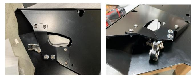
Rear Door Latch Installation Pictures. Use 6mm bolts and washer for latches only. Use ¼" bolts for mount plates.
