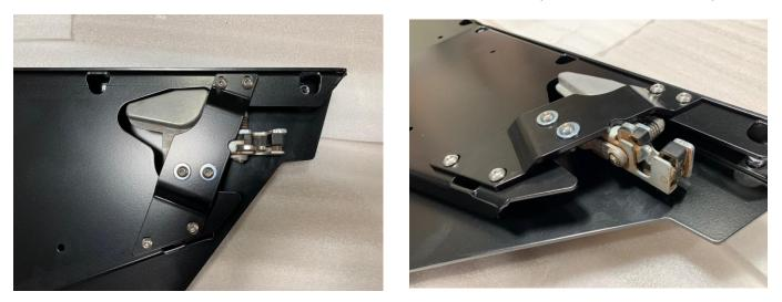
Take notice of the direction of the bends on the door latch mounts. There is adjustment in the holes on both the plates and the latch mount holes. Make final adjustments when installing on machine.
