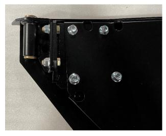
Step 4. Install the front latch plate and factory latch as shown below. Use 1/4 bolts, washers, and nuts for the latch plate. Use M6 bolts for the factory latch. The M6 bolts should be in their own labeled baggie in the hardware bag.
