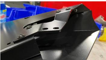
**Step 5**. Carefully intall door using the large 1/2" bolt with a lock washer and Flat washer installed on the bolt (put lock washer on bolt first, then flat washer.) Slide door hinge into mounting bracket on RZR.
