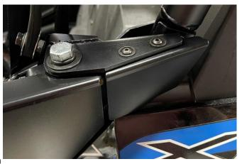
Step 7. Install hinge cover using the \( \frac{1}{4} \)" bolts. Test for interference from door when opening before tightening.
