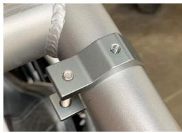
**Step 3**. Place windshield on cage and clamps. move clamps to line up with holes on windshield frame. Use the 1/2" long holts and flat washers
