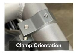
**STEP ONE** – Clip the billet mounts into approximate positions onto roll cage as shown in picture. Use 2" long bolts to hold clamp in place. Only tighten Bolt enough to hold clamp in place but still moveable.
