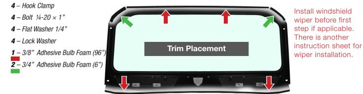
**STEP ONE –** With the windshield laying on its front place the large bulb adhesive trim on the two top corners as described in the figure above. The smaller bulb trim will be used along the center top and the bottom of the windshield frame. **Take your time applying the trim. The adhesive on the trim is extremely powerful and it will not release once applied.**
