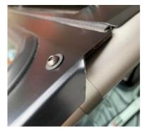
**STEP ONE** – Clip the billet mounts into approximate positions onto roll cage as shown in picture. Use 2" long bolts to hold clamp in place. Only tighten the bolt enough to hold clamp in place but still moveable.
