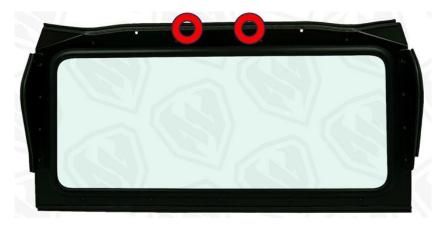
**Step One:** Remove any roof on the machine. If using the OEM plastic roof, the bulb seal along the top of the windshield will need to be cut to allow room for the factory roof clamps to go through the notches in the windshield. Approximate location shown circled in red above.
