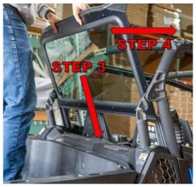
bent side of the clamp on the rear. Bolt it in with the 1" bolts, locknuts, and washers on both sides. The bulb seal along the top might need to be trimmed to make room for the bolts. Bolt the lower brace to the clamps using the 2.5" bolts and both types of washers.
